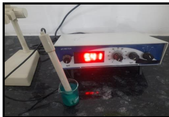
Fig.3. Determination of pH-by-pH meter and pH paper
